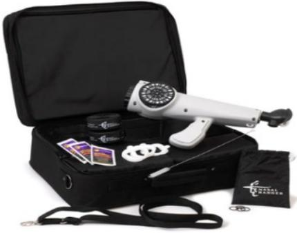
*The olfactometer will allow inspectors to quantify odors.*
