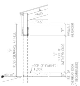
"D" = Bottom elevation (B.E.) of overhead door: **0' 4"** The bottom of all overhead doors (top of finished floor) are recommended to be placed at 4" above the 100'-0" mark (100'-4"). In building without paved floors, B.E. of doors may be lower - e.g. 100'-0".
