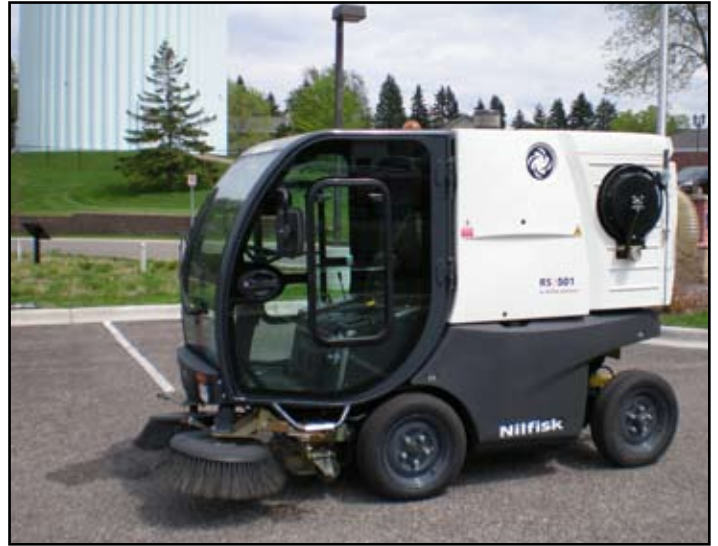
Routine maintenance of porous pavement includes vacuum sweeping at least twice a year.
