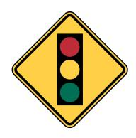
ASWS include the yellow signs stationed over the roadway that often feature flashing yellow lights to warn of a traffic signal ahead.
