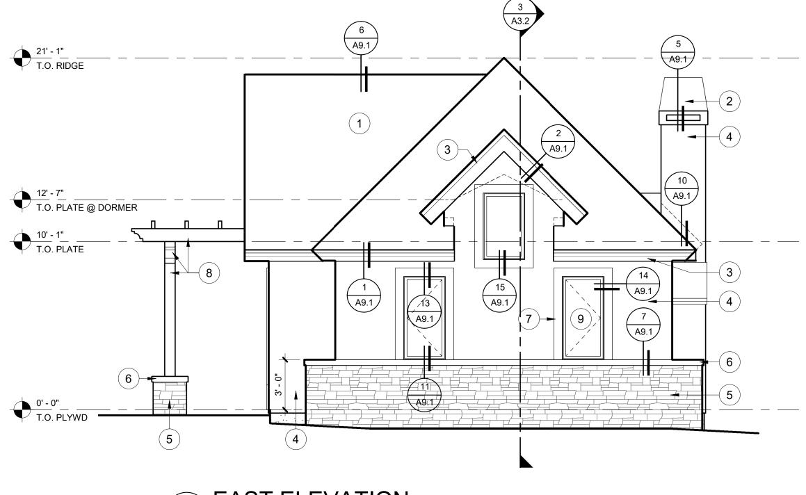
4 EAST ELEVATION A3.1 SCALE: 1/4" = 1'-0"
